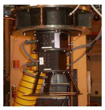
Calibration and polarimeter module at the Cassegrain focus.
