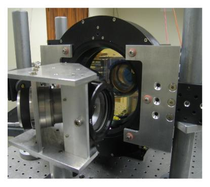
The Image Stabilizer Unit delivered by the Laboratoire d'études spatiales et d'instrumentation en astrophysique in May 2004 on the test bench with a simulated laser star at the CFHT.
