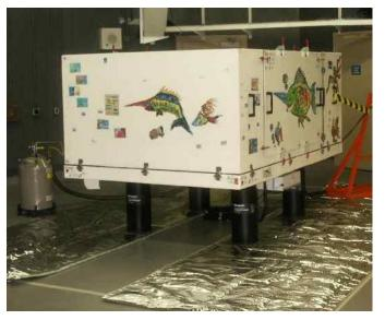
The spectrograph in its thermal enclosure.
