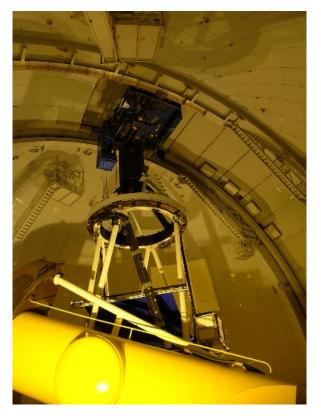
WIRCam being mounted at the telescope with the upgraded upper end and prime focus cage.
