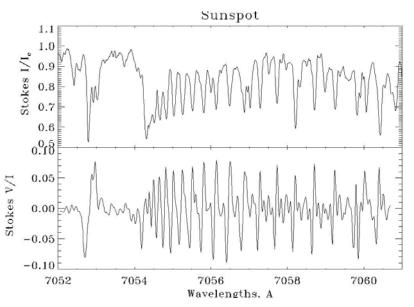
Part of the spectra of a solar sunspot between 705 and 706 nm. The top panel shows the intensity of the light in the molecular TiO line. The bottom panel shows the circular polarization, Stokes V; the pattern is caused by the presence of a magnetic field inside the sunspot.
