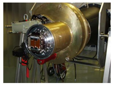
The mosaic is now in place on the back of the cryostat
