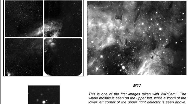
This is one of the first images taken with WIRCam! The whole mosaic is seen on the upper left, while a zoom of the lower left corner of the upper right detector is seen above. On the left, a star from one of the corners is highly magnified, demonstrating the high optical quality of WIRCam. The seeing was good enough to show the undersampling of the image due to the 0.3" pixels...
