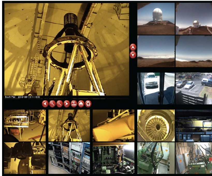
Figure 1 Replacing the eyes and ears of the Observing Assistant is one of the key-components of the OAP environment. Fixed or remotely controlled cameras at strategic locations offer enough information for a close look at the critical components of the observatory and for well-informed decisions from remote location (from the Waimea headquarters to mobile devices).
