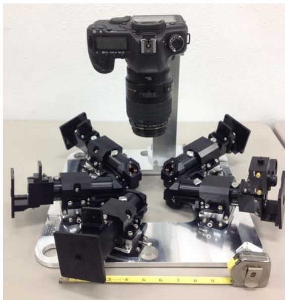
Figure 17 – The mWFS assembly in the lab at MKIR in Hilo is shown. The assembly consists of 5 high order/speed wavefront sensors and a commercial camera for acquisition purposes.
