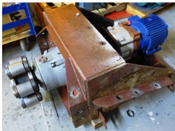
Figure 10 - A shutter drive unit showing, from left to right, the pinion roller assembly, the 319:1 speed reducer, the red steel unit frame, the brake and 5 hp drive motor.
