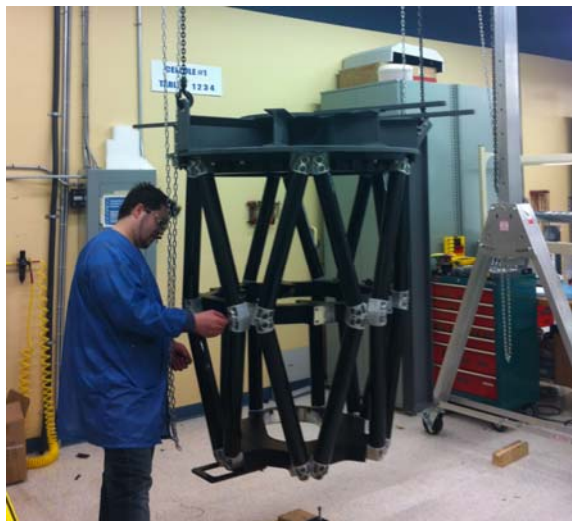
Figure 14 - The main SITELLE instrument structure during assembly at ABB. The truss members are stiff, light weight carbon fiber tubes.
