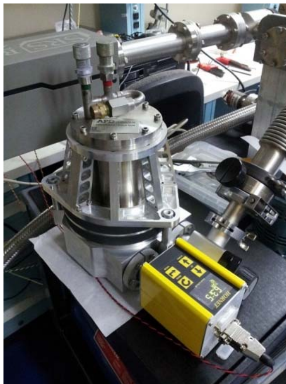
Figure 15 – A fully assembled SITELLE science detector dewar is shown undergoing vacuum testing.
