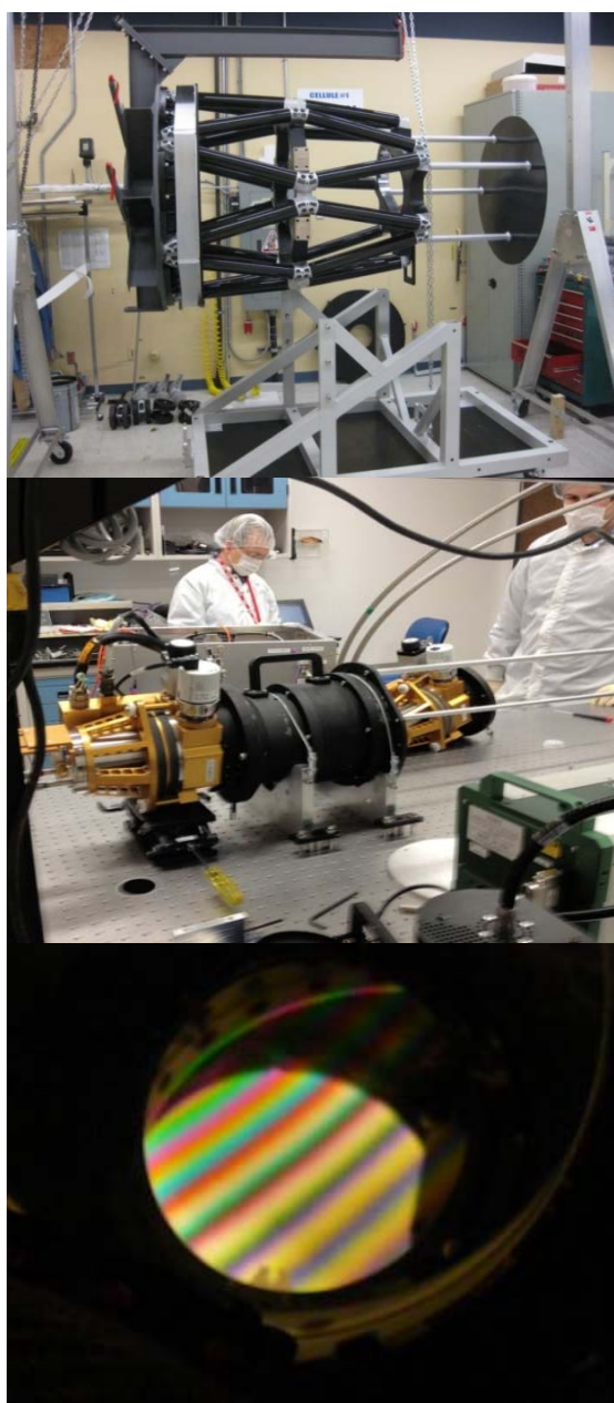
Figure 14 – Top: The carbon fiber superstructure of SITELLE is shown in ABB's lab. Middle: CCD camera integration at the University of Laval is shown. Bottom: White light interference fringes from SITELLE's beam splitter are evident.
