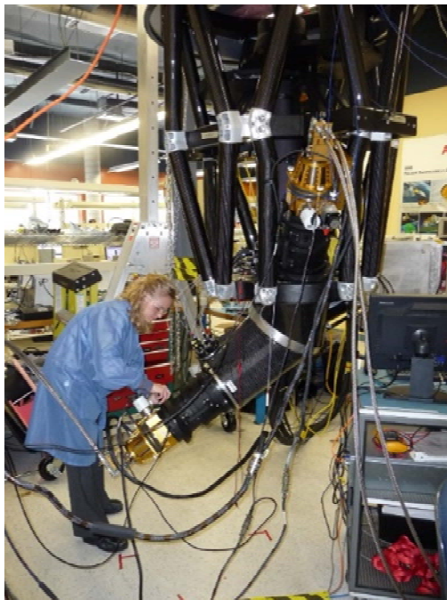
Figure 15 – SITELLE is shown in the lab at ABB, where it is being built. The black carbon fiber structure supporting the embedded interferometer is evident, as well as the pair of CCD systems (gold dewars) at each end of the interferometer.
