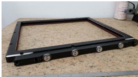
Figure 13 – Bearings retrofit into the MecaCam filter frames now provide a near-zero friction mechanism, leading to more reliable and safer filter exchanges.
