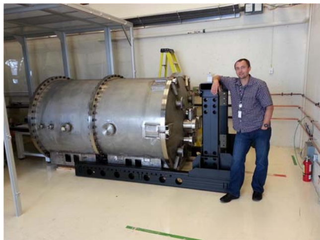
Figure 9 – Above: the lower and upper parts of SPIRou's Cassegrain assembly are shown. Below: The large cryostat that will house SPIRou's spectrometer is shown.
