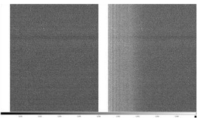
Figure 10 – Image after subtraction of a master bias image (left) and a raw bias image (right). Notice the removal of residual "waves" in bias in the columns initially read out.
