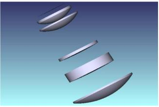
Figure 17 – Prime Focus Corrector and ADC for MSE.
