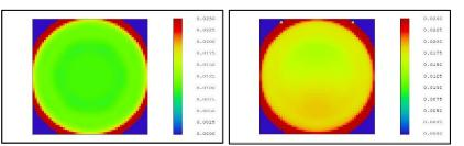
Figure 16 - RMS image quality maps for (left)  $ZD=0^{\circ}$  and (right)  $ZD=50^{\circ}$ . The asymmetry in the  $ZD=50^{\circ}$  case is due to the ADC action.
