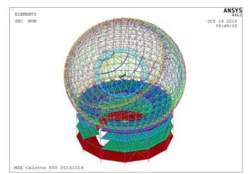
Figure 18 - EDS Calotte FE model.
