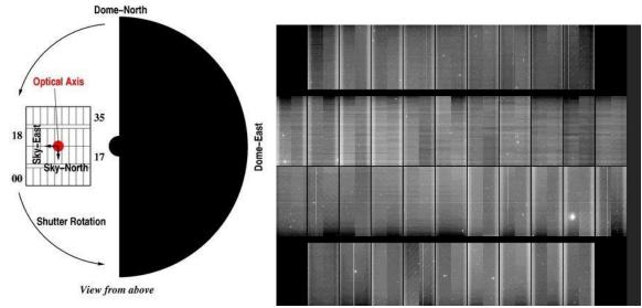
Figure 16 - Left: Schematic of MegaCam shutter. Right: MegaCam Exposure binned by a factor of 24 to illustrate the occasional noise patterns visible on CCDs in the second row.
