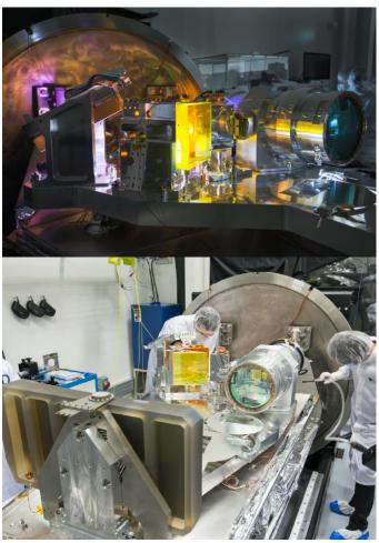
Figure 12 – The opto-mechanical bench of SPIRou's spectrometer is shown prior to being sealed, pumped, and cooled.
