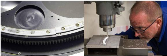
Figure 20 – Left: Image showing some of the damaged sapphire balls in the lower filter wheel prior to removal. Right: Careful machining of new Teflon spacers.
