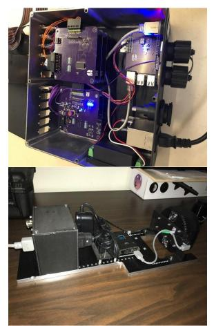
Figure 23 – Top: TCS RBUSS replacement hardware is shown. Bottom: New TCS Cassegrain CCD guide camera and mount, ready to be deployed on the summit, is shown.
