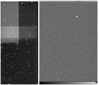
Figure 17 – Left: A binned image of Chip 12 displaying the increase in background across several rows. Less than 1% of images are affected by this issue. Right: Vertical 2-4 pixel features we coined raindrops. These affect ~50% of MegaCam images and have been present in the data since MegaCam was commissioned. Their frequency has not increased over time and they are uniformly distributed across the focal plane.
