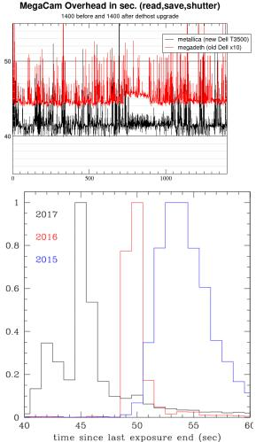
Figure 15 – Top: The x-axis shows the number of exposures tested and the y-axis gives the total overhead time before (red) and after (black) upgrades, including reading, saving and shuttering. Bottom: Histograms (as of Sept 18, 2017) of dead time between all exposures archived at CADC during 2015 (blue), 2016 (red) and 2017 (blue). Figure courtesy S. Gwyn.
