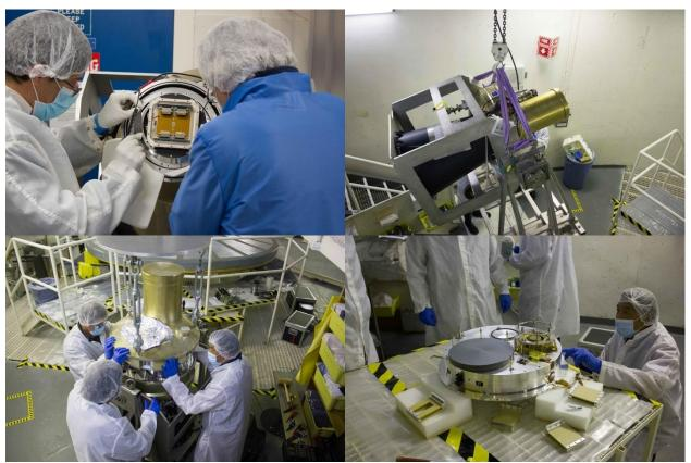
Figure 19 – Top: Removing detectors from WIRCam and lowering WIRCam to the floor of the aluminizing room for final disassembly. Bottom: Disassembly of WIRCam in the aluminizing room and the filter wheel assembly by itself.
