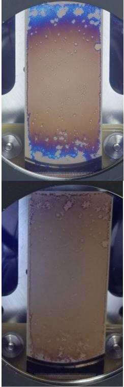
Figure 22 – Before (top) and after (bottom) pumping on the dewar, as described in the report, left a significant reduction in surface contamination.
