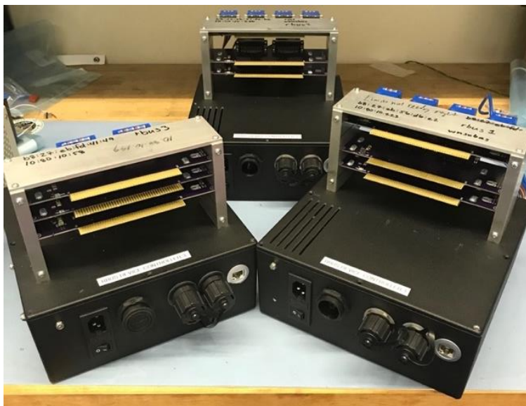
Figure 23 - Three RBUS device controllers have been fabricated and are ready to deploy.
