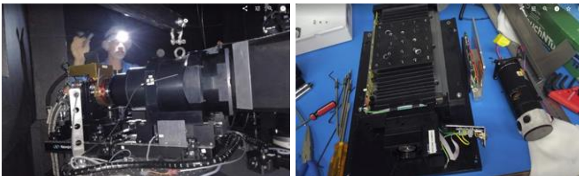
Figure 18 - (Left) Focus stage with camera optics on top within the ESPaDOnS enclosure. (Right) ESPaDOnS focus stage removed and disassembled for repair.
