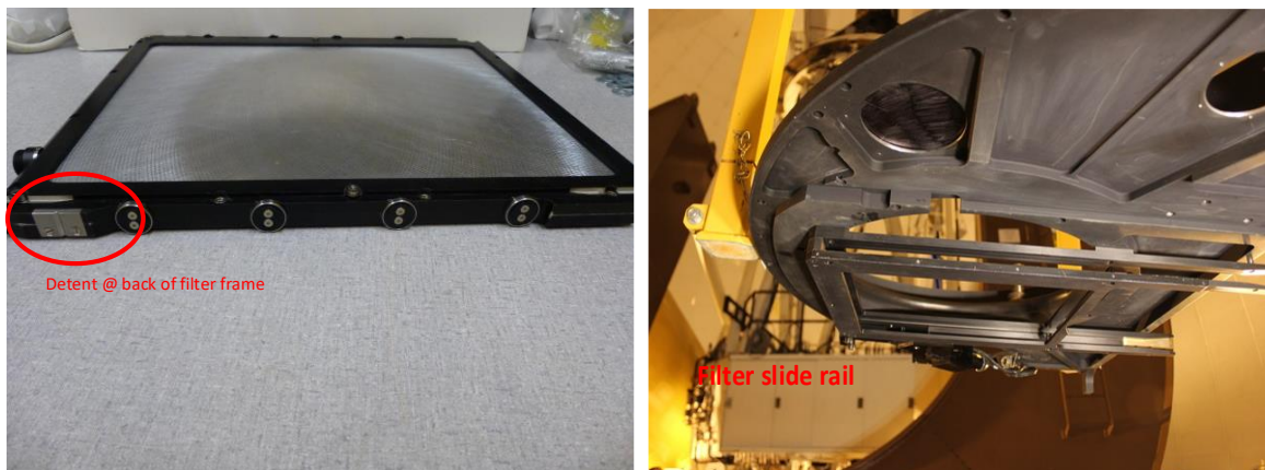
Figure 17 - (Left) The detent is used to lock the filter in its jukebox slot. Two counter-sunk, stainless steel screws hold the detent in-place. (Right) The slide rail is mounted on the superior plate and can only be accessed by first removing the MegaCam cover, camera and supporting structure.
