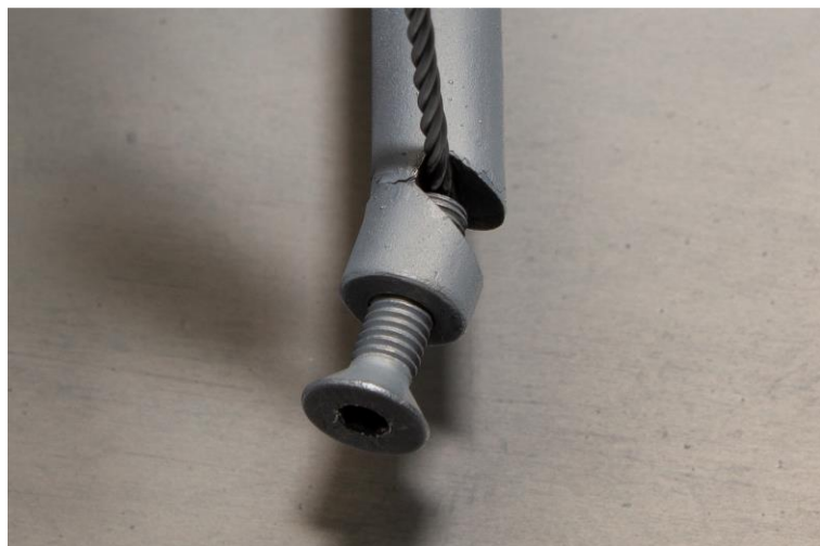
Figure 24 - Original electrode design. A crack is visible at the cusp.
