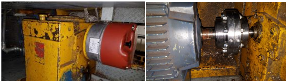
Figure 19 – DeMag motor, Gearbox, and Stearns Brake (Left). New motor/gearbox coupler (right).
