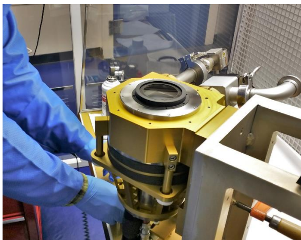
Figure 10 - Field flattening lens being installed as a replacement for the cryostat window in the clean room.
