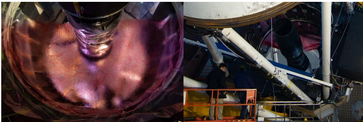
Figure 26 – First Contact applied to the primary mirror prior to peeling (left) and after peeling (right).
