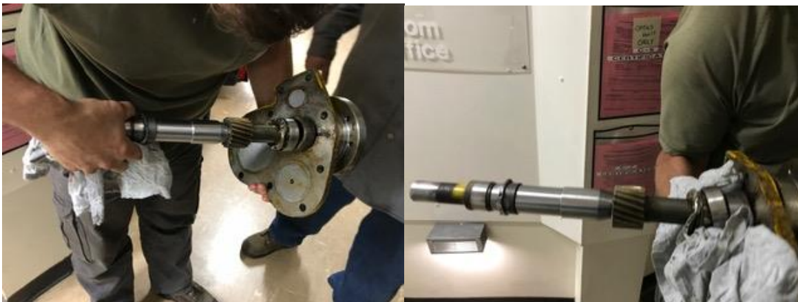
Figure 20 – Damaged drive shaft and bearings shown removed.
