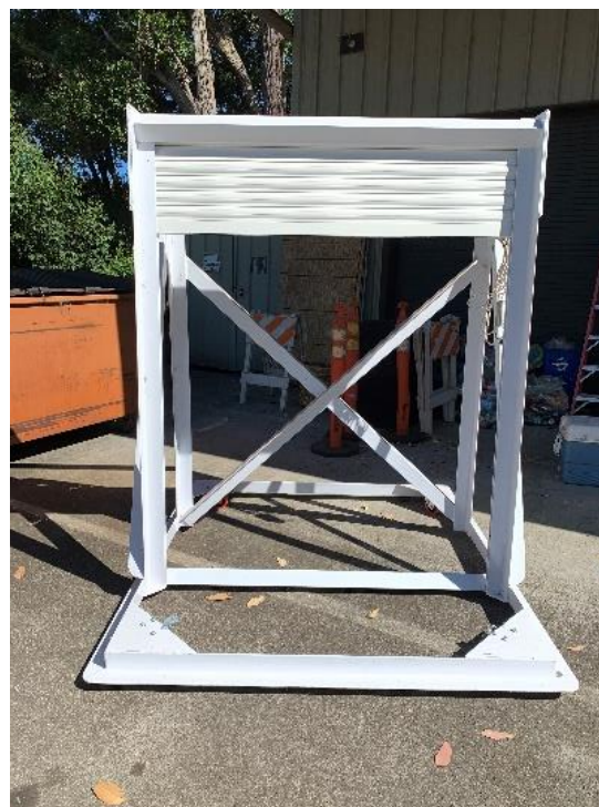
Figure 21 - Scaled down dome vent test fixture.
