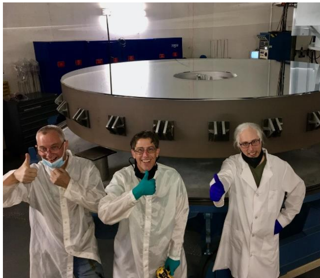
Figure 7 - A happy coating team shows off a freshly coated primary mirror. Due to improvements in the coating chamber, the coating thickness for this runs exceeds all previous coatings by \sim 30\text{-}50\% .
